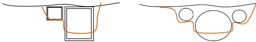
Illustration 2a. Using elevated equalizer culverts to capture excess flows once bankfull flow is exceeded.
