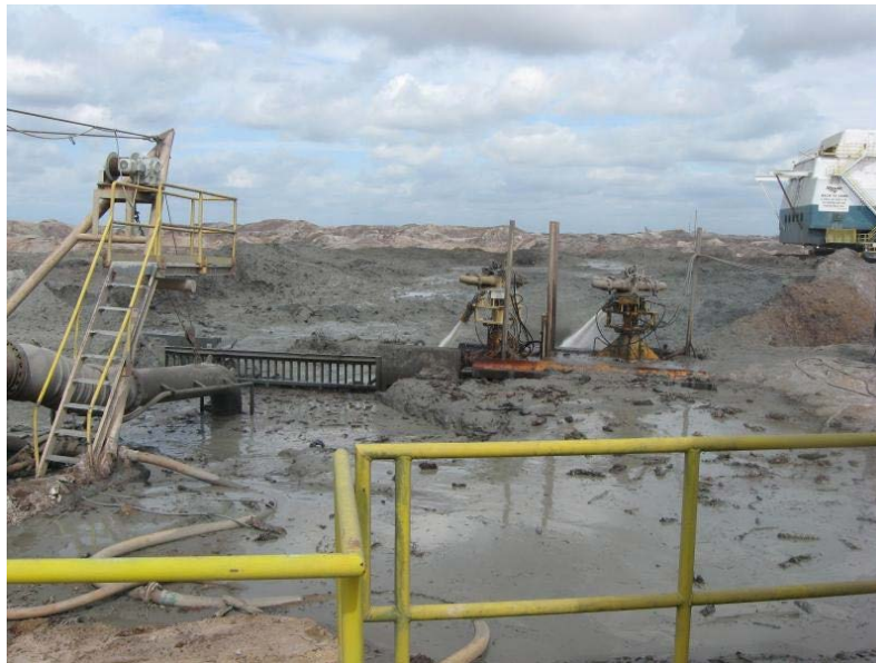
High pressure water jets used to create a slurry for transportation of phosphate matrix from field to separation plant
