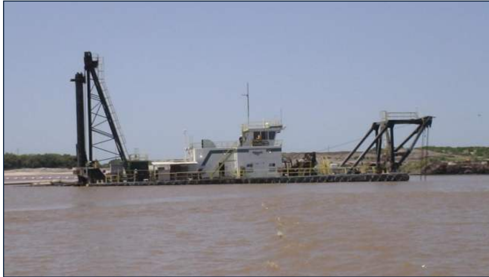
Figure 2-7. Dredge-Based Phosphate Mining at the Wingate Creek Mine
