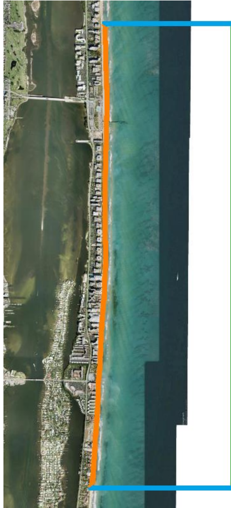
Figure 3-3. BOUSS-2D boundaries - wavemaker (green), sea sponge layer (blue) land sponge layer (orange).
