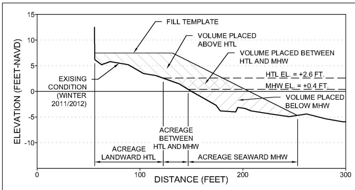
Figure 2-1. Schematic of construction volume and acreage estimates.
