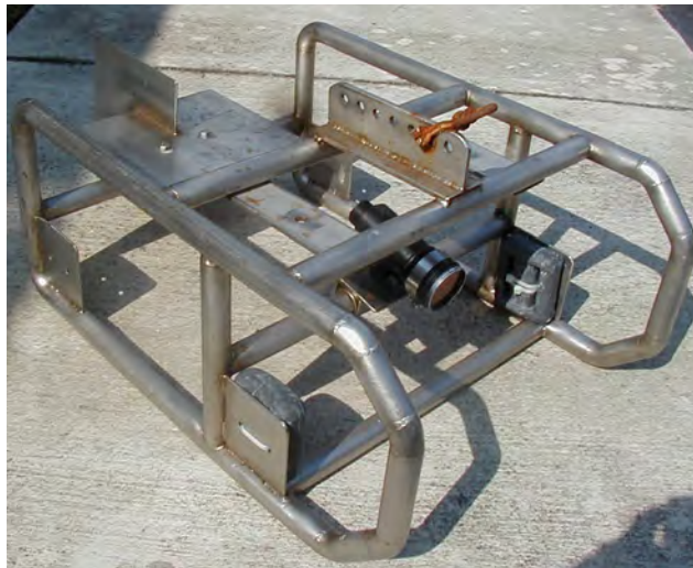
Photograph 1 Towed video camera and sled used for mapping and assessment of marine resources offshore Pinellas County
