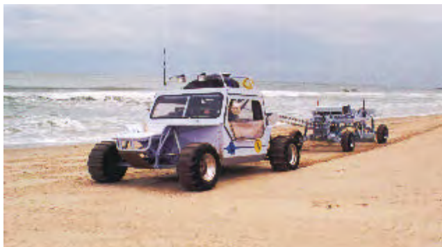
Figure 8. The MTADS vehicle is shown conducting a magnetometry survey south of Round Island Park.
