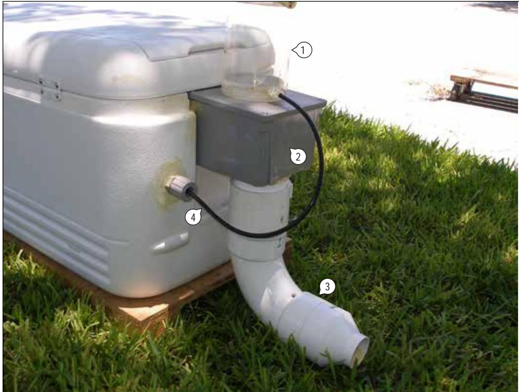
1. Multiprobe flow cell for monitoring pH, temp, ORP of GW leaving the SS flow-through chamber
