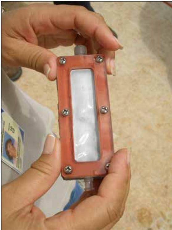
Figure 1-2. A completed diffusion chamber.
