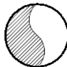
CYLINDER BREAK LINE PARALLEL TO VIEWING PLANE
