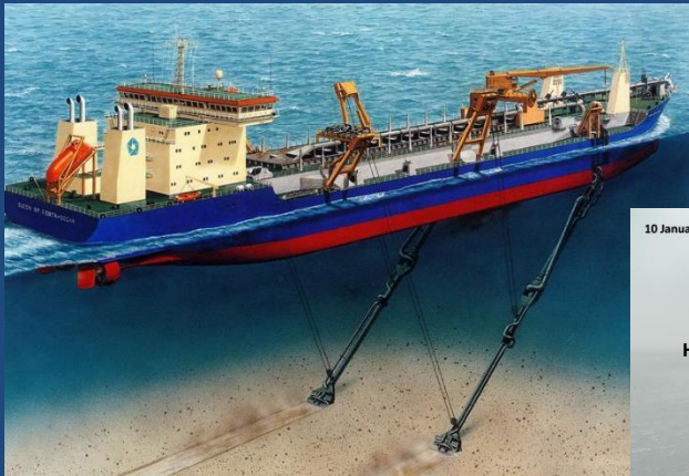
Hopper dredge loading sand from seafloor
