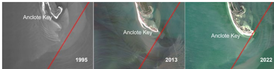
Figure 1-3. Maps of Anclote Key and the federal channel from 1995, 2013, and 2022 showing the migration of Anclote Key across the federal channel (original Cut 2) and the need for the 2023 realignment.
