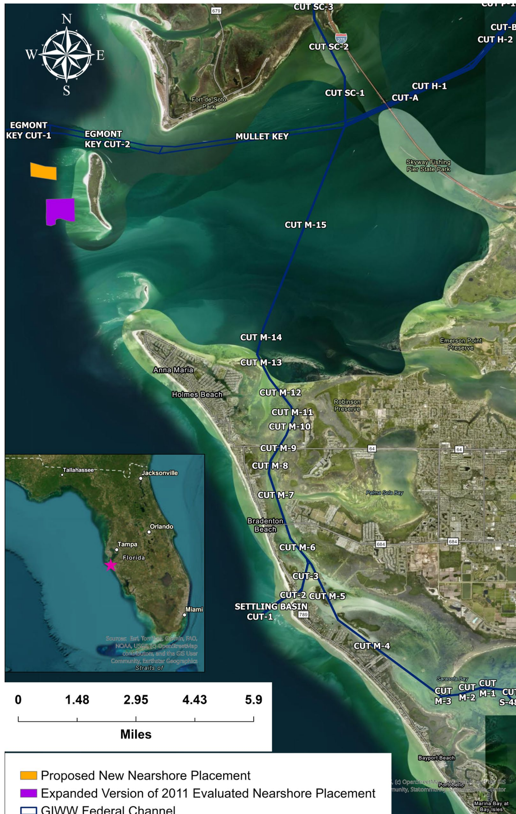
Figure 3-2: Expanded Version of Previously Evaluated Nearshore Placement and Proposed New Site for Nearshore Placement at Egmont Key
