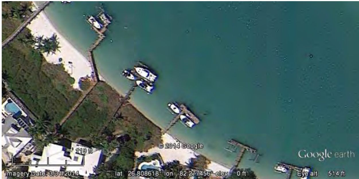
Figure 3. The image above shows an example of dock shapes including a T-shaped and L-shaped (©2014 Google)
