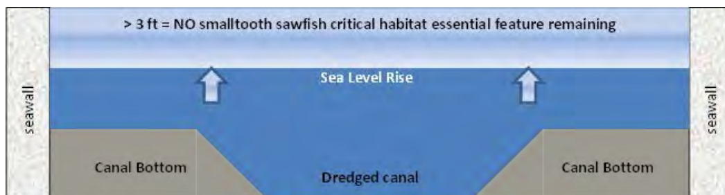
Figure 31. Diagram A depicts a cross section of a historically dredged channel/canal within the boundaries of the critical habitat units that has not been maintained. Diagram B depicts the typical cross section of a maintenance dredged channel/canal. Diagram C depicts a cross section of a maintained dredged channel/canal after sea level rise of > 1 ft.
