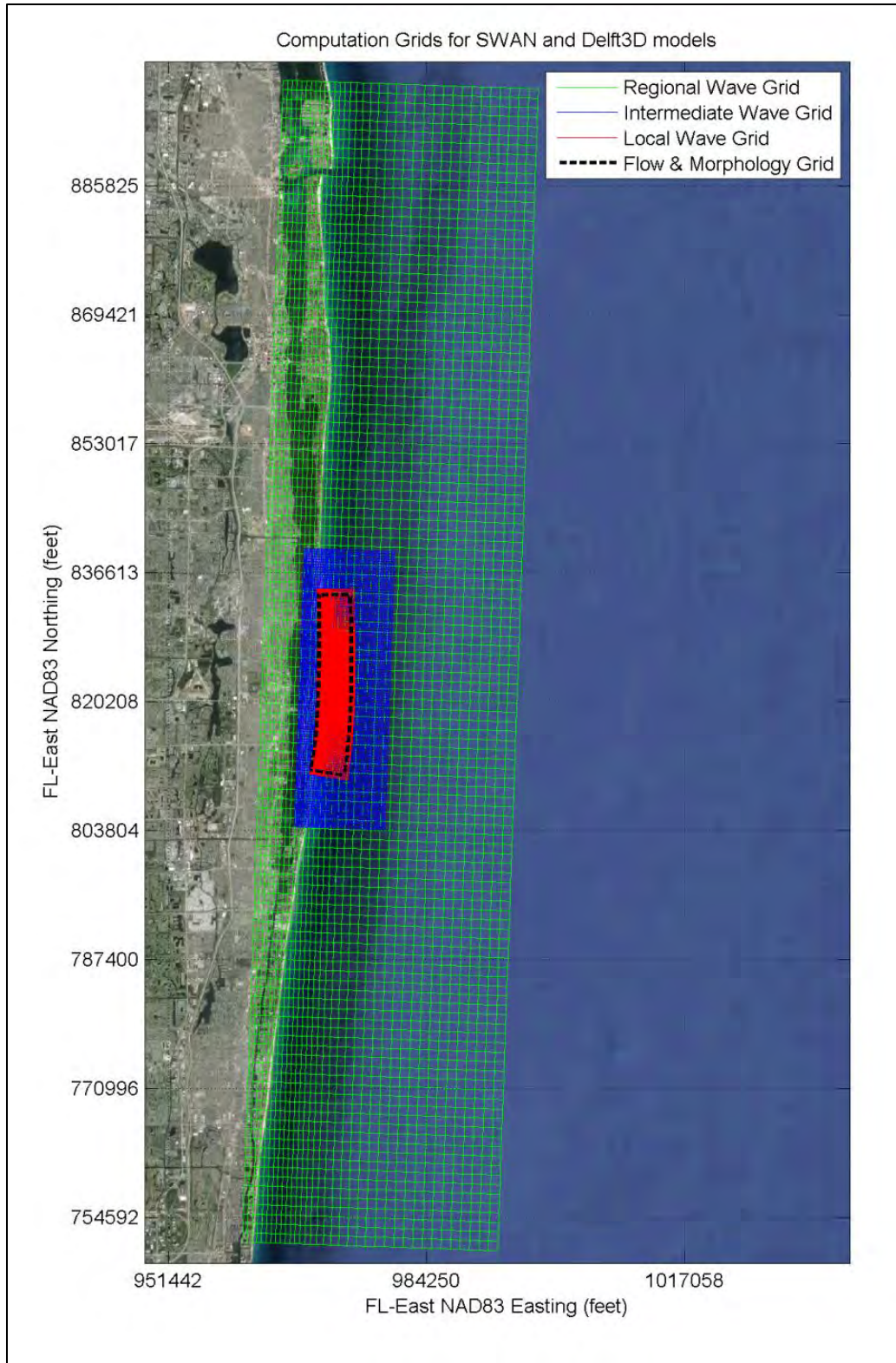
Figure 3-1. Computational grids used in Delft3D-WAVE and Delft3D-FLOW calibration and production runs.
