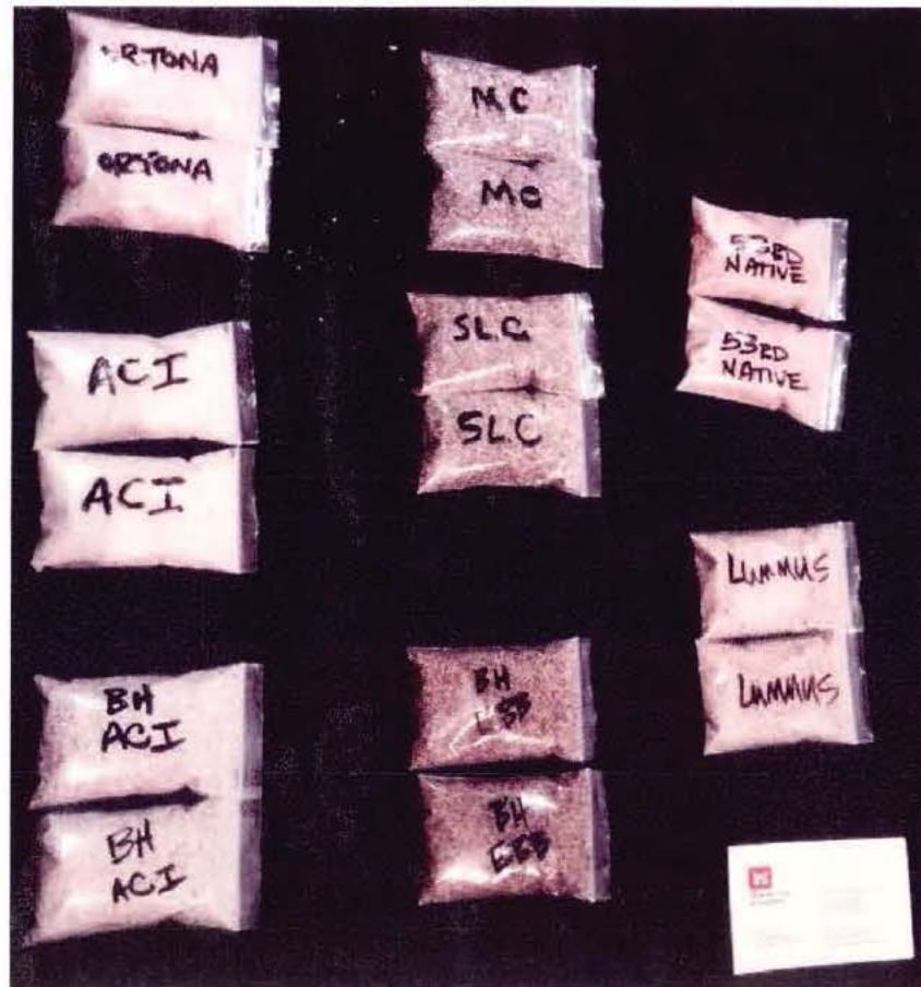
Figure 51 - Comparison of Native Miami-Dade Beaches to Other Sand Sources (53 rd Street Native; MC = M4-R105; SLC = SL10-T41; Lummus = Lummus Park; ACI = ACI mine; Ortona = Ortona mine; BH Ebb = Bal Harbor Ebb Shoal).
