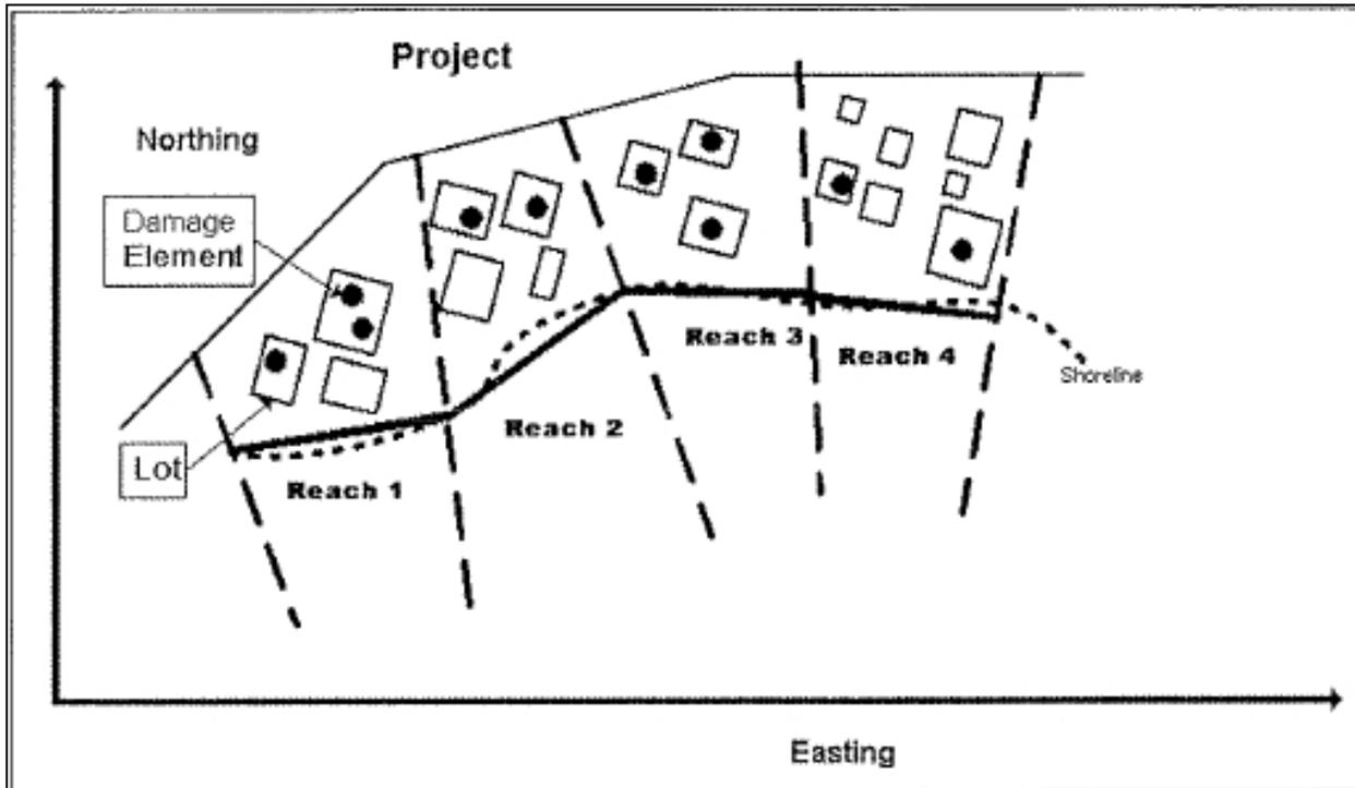
Figure A - 14. Beach-*fx* model setup representation.
