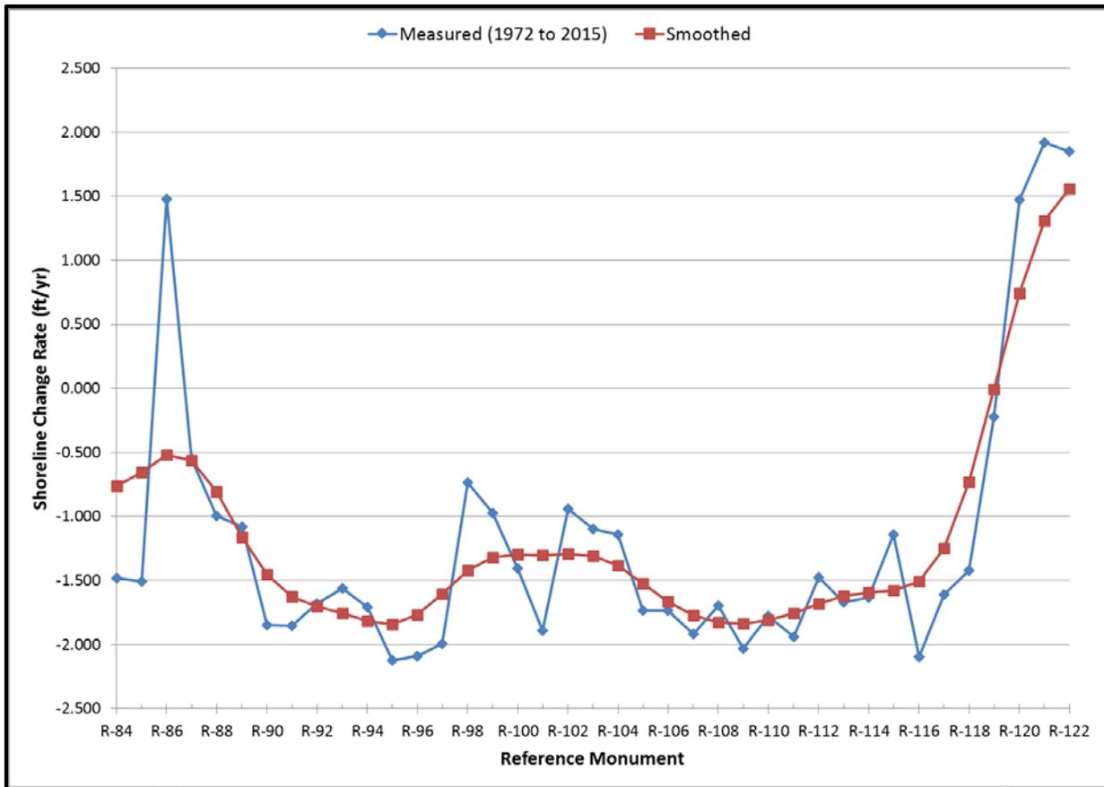
Figure A - 26. Target MHW shoreline change rate.
