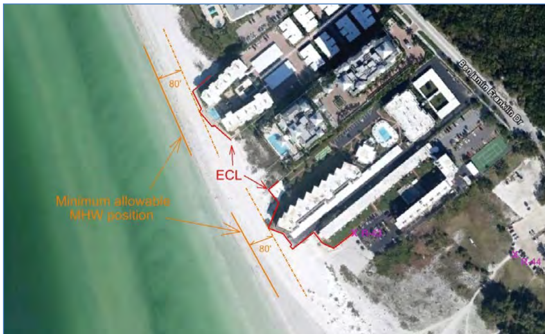
Figure 2. Minimum required shoreline positions along southern Lido Key.
