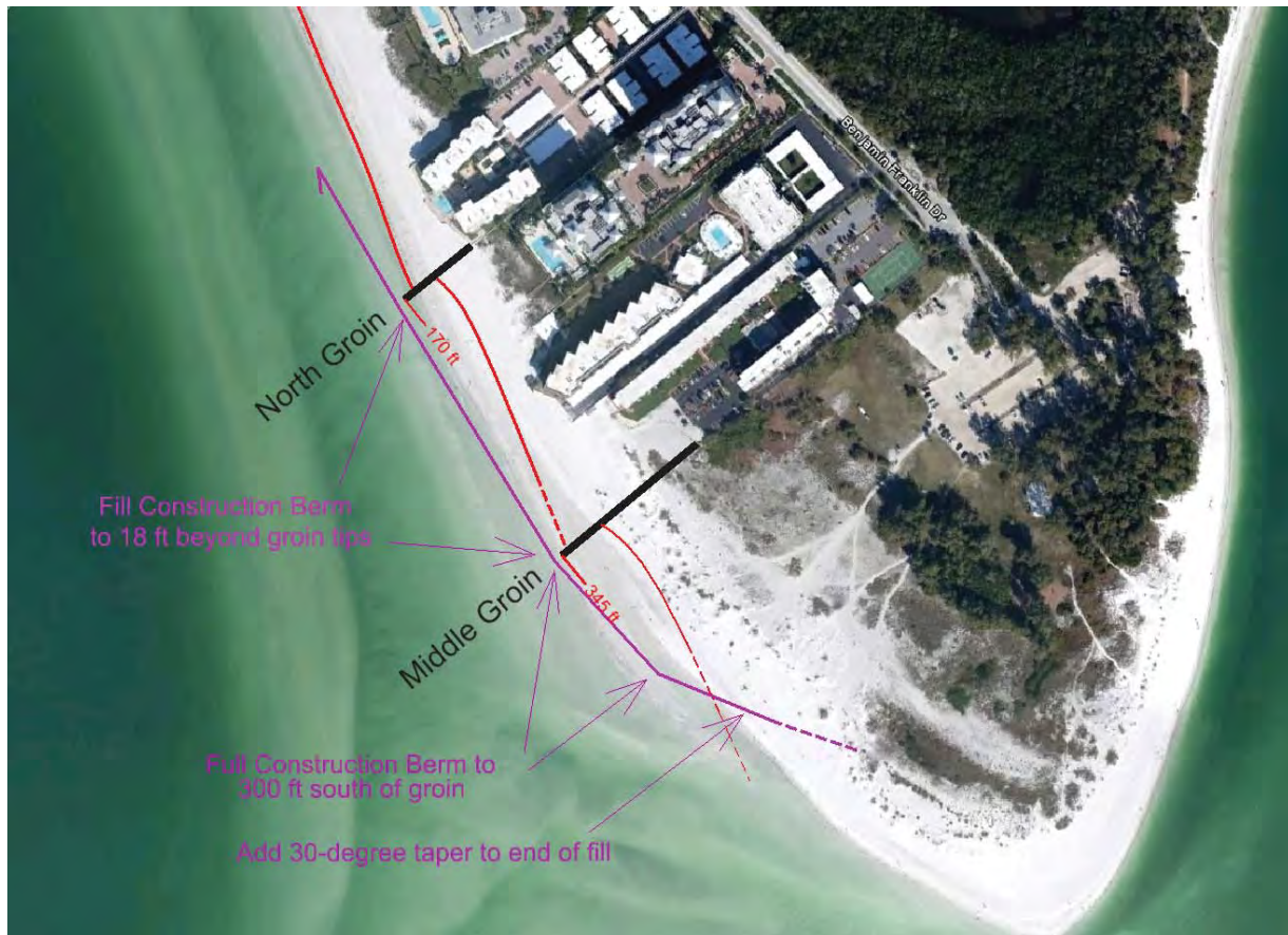
Figure 4. Final recommended plan showing the locations of the two groins and proposed beach fill at the southern portion of the island.
