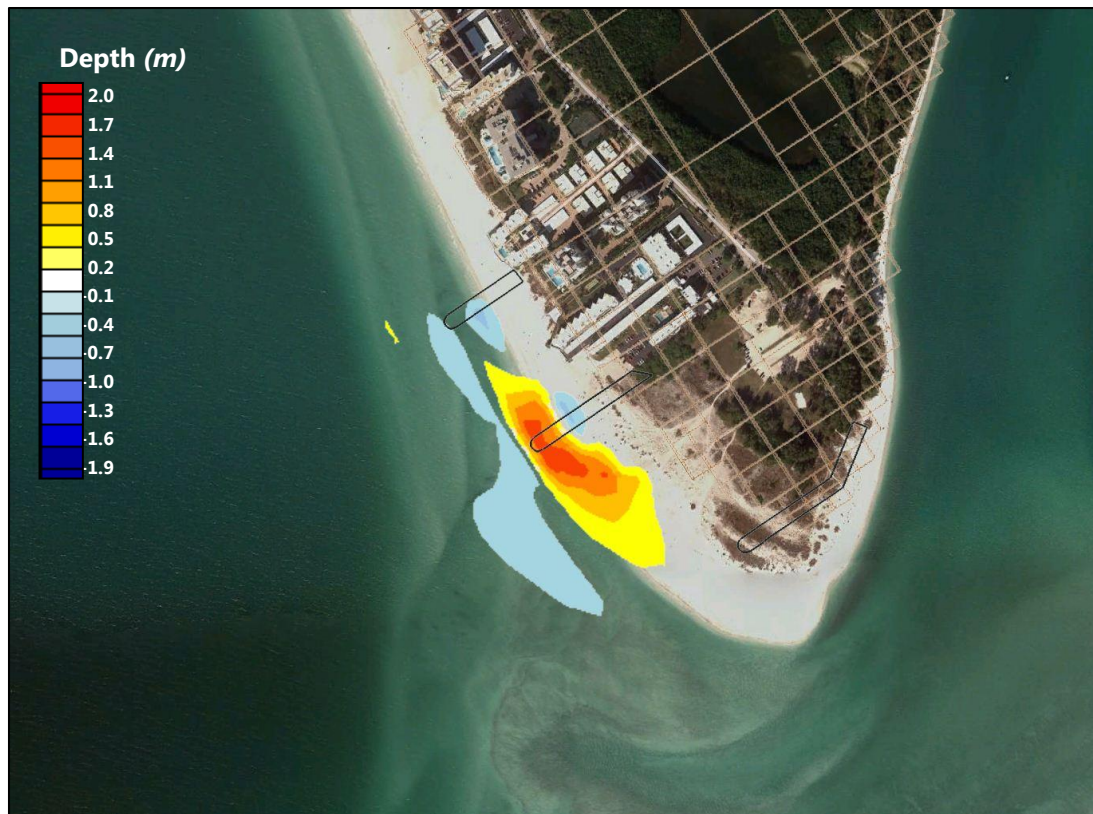
Figure 97: Groins with nourishment; Ending morphology difference for six month run 2004 = (groins were in place with beach nourishment) – (no groins with beach nourishment)
