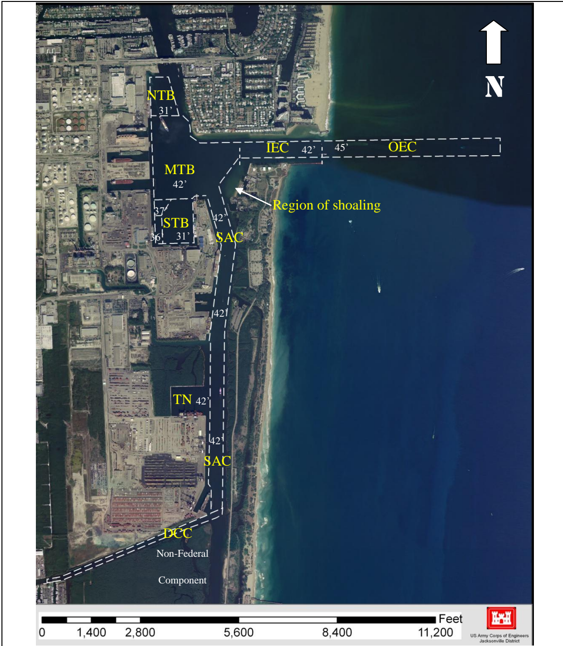
Figure 1: Existing Federal Channel Components
