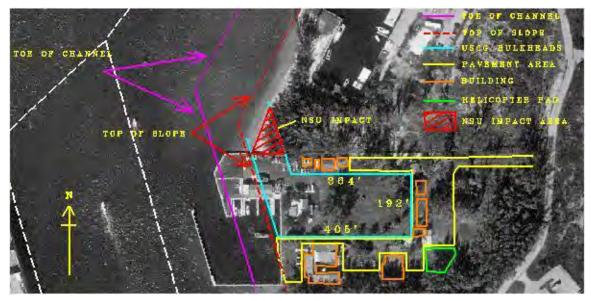
Figure 12. USCG Basin Relocation Plan
