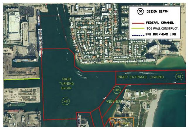
Figure A- 78. Toewall and EFB Locations (Conceptual) – North Selected Plan
