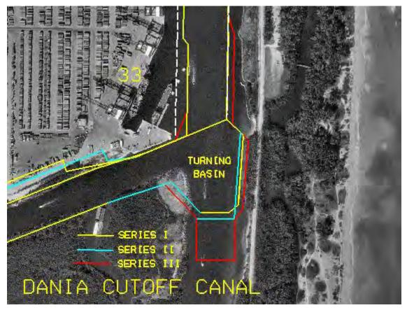
Figure 17. Modification of Dania Cutoff Canal for Series III Simulation
