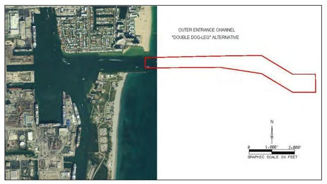
Figure A- 14. OEC – Double Dog-Leg Alignment (1)
