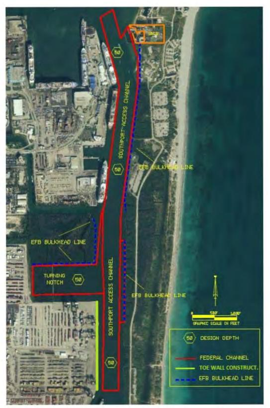
Figure A- 79. Toewall and EFB Locations (Conceptual) – South Selected Plan
