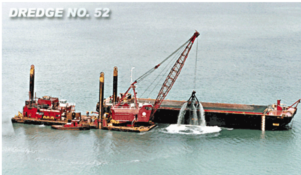
Figure 6. Clamshell Dredge (left) with Scow (right). Photo courtesy of Great Lakes Dredge & Dock Company.
