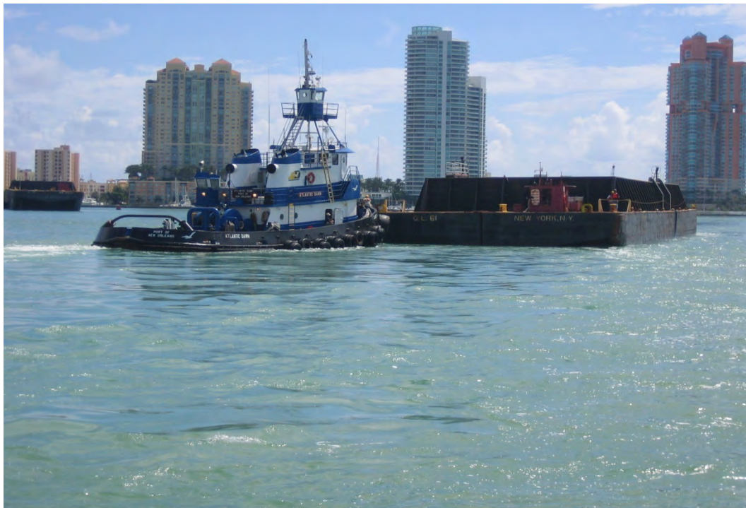
Figure 8. Split hull barge being pushed by tug.
