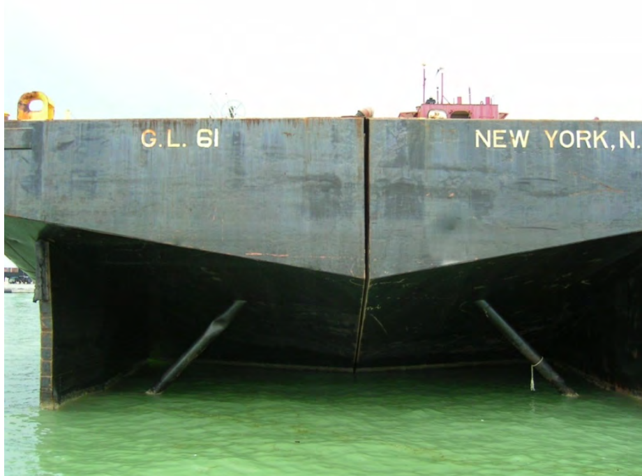
Figure 9. View of stern of split-hull scow.
