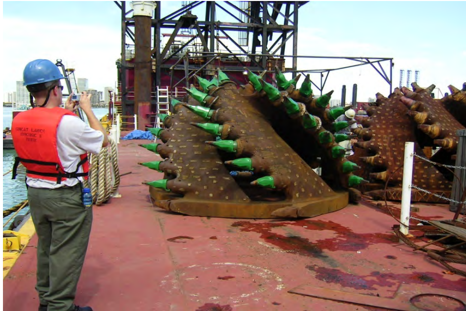
Figure 5: Typical large cutterhead.
