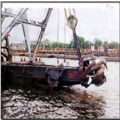
Figure 4: Cutterhead pipeline dredge schematic and representative close-up photographs (photo/drawing: Engineer Research and Development Center, 2007).
