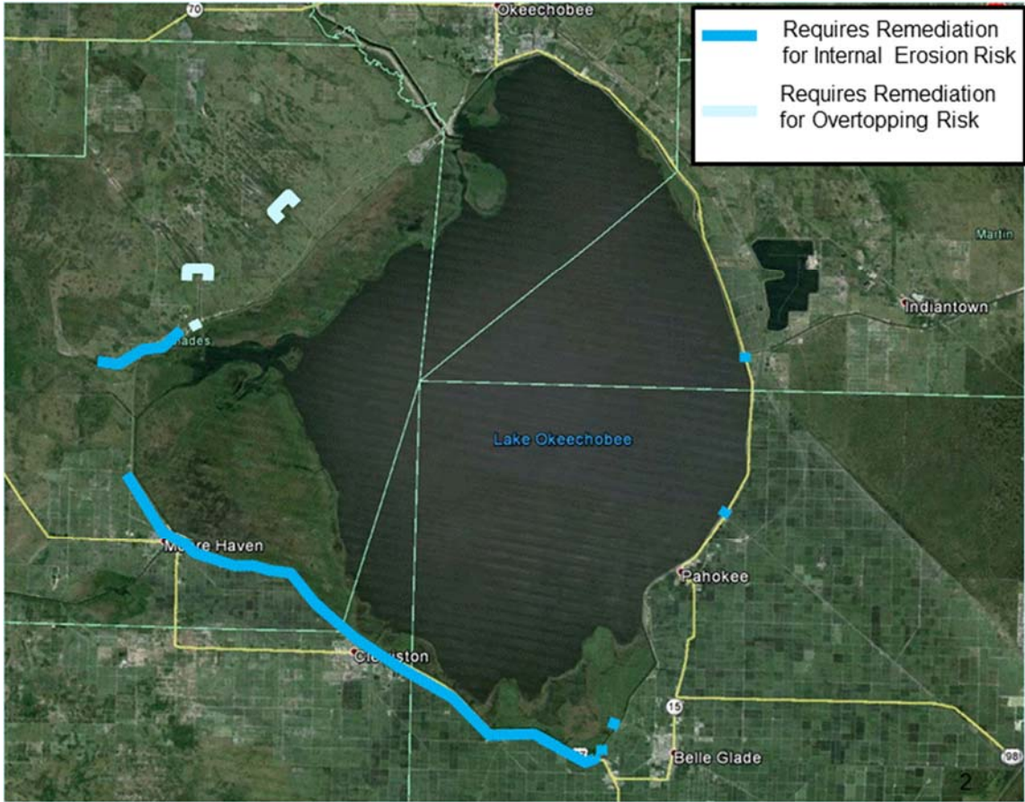
Figure 1-5: This figure portrays the locations where risks have been identified as intolerable due to combination of high probability of failure and the consequences of a failure.
