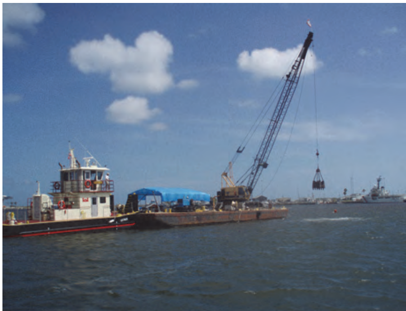
Figure 5. Bucket dredge equipment used in simulated operation.
