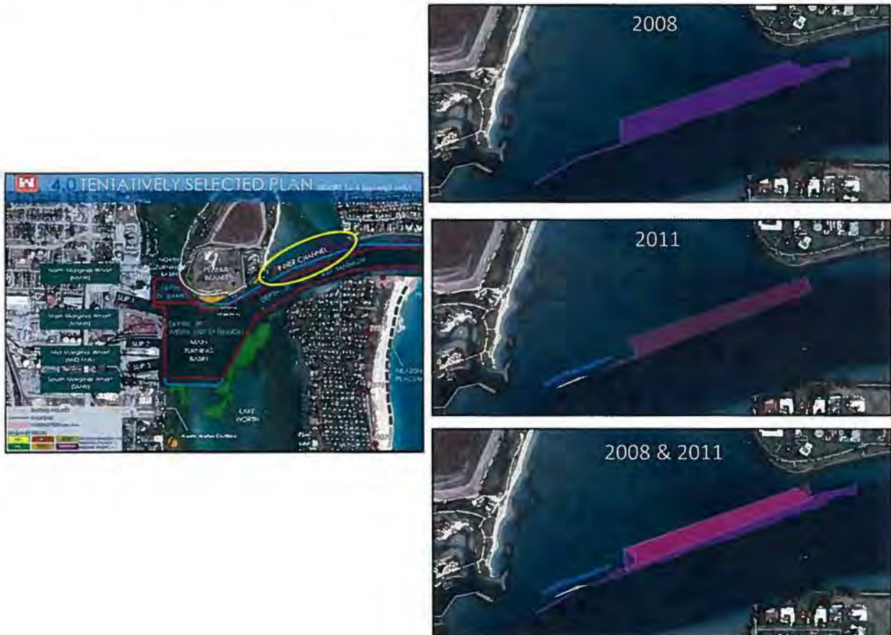
Figure 3: Hardbottom exposure along the northern edge of the inner channel. The image on the left is modified from figure ES-2 in the EIS. The area circled in yellow and hardbottom exposure cover is illustrated in the images on the right. The top right image is hardbottom reported in this area in PBS&J 2009 (4.2 ac); the middle image is from DC&A 2012 (3.2 ac); the lower right image depicts cumulative hardbottom exposure (4.6 ac) in this area.
