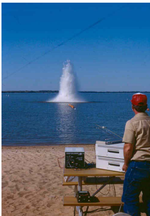
Figure 6 Unconfined Blast of Seven Pounds of Explosives
