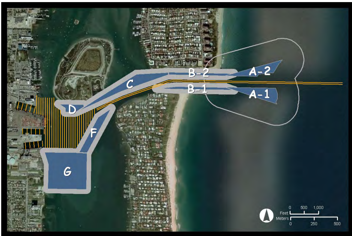
Figure 1. General location map for the Environmental Resources Report study area. Diver-investigated zones A-1 thru G (blue) with a 150-ft buffer (gray). Note the offshore 750-ft buffer (A-1 and A-2). Towed-video transects through the federal channel, turning basin, and existing berths are depicted in gold.
