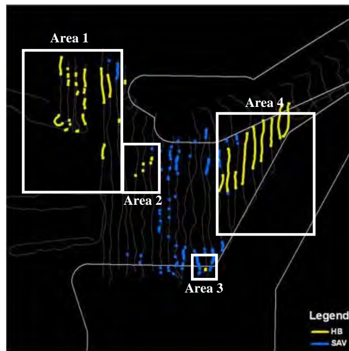
Figure 22. Four areas of hardbottom located in the turning basin.
