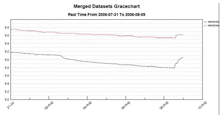
We can see the 250 cfs pumping which began on 2006-08-02 at 16:00 flattened out the NESS20 SW and we can see the pull on the aquifer by the canal. This is the water level in the aquifer plotted with the water level in the marsh.
