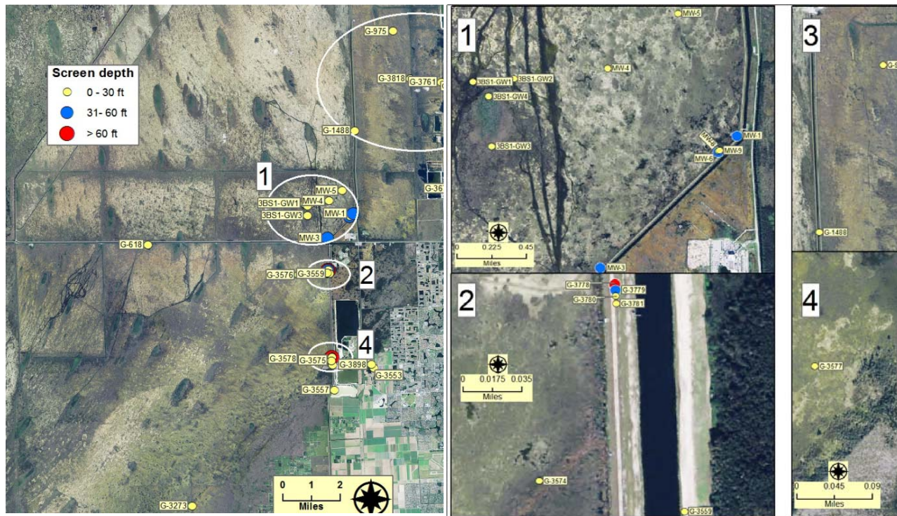
FIGURE C.1-6. Wells sampled for water quality are a subset of the groundwater flow and level monitoring network. All groundwater quality data compiled during the Increment 1 test will be incorporated into the source water characterization and water budget tasks. Groundwater quality
