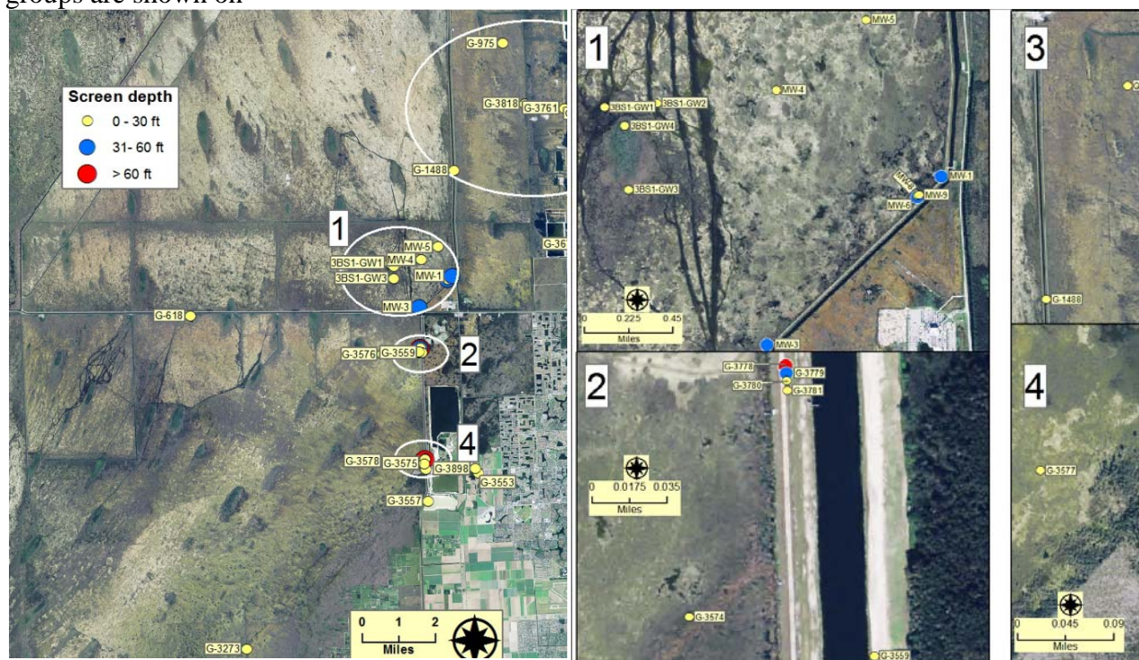
FIGURE C.1-6. Groundwater level and flow data at monitoring locations in WCA-3B and along L30 ( FIGURE C.1.6-1 ) will characterize seepage in upgradient and background positions, and also will define the S356 zone of influence north of the pump station. Groundwater level and flow data obtained in northern NESRS and along the northern and southern portions of L31N ( FIGURES C.1.6-2 and C.1.6-4 , respectively) will characterize seepage in downgradient positions, and also will define the S356 zone of influence south of the pump station. Hydrologic effects of the MDLPA seepage barrier along L31N also will be evaluated from these data.
