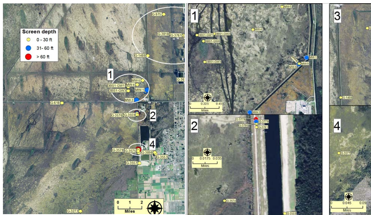
FIGURE C.1-6. The result is a comprehensive groundwater monitoring network that will provide detailed data to evaluate effects of S356 pump station operation. TABLE C.1-2 lists monitoring wells and clusters by location, and the types of data that are measured at each well. All wells listed in TABLE C.1-2 will be evaluated during the first few months of the Increment 1 test. Hydrologic responses to S356 pumping stresses in surrounding monitoring wells will be reviewed in context of seasonal water level changes and other distal pumping stresses (mining operations or MDWSD northwest wellfield) before deletion from the monitoring program. Those wells that show no response to S-356 operation will be deleted from the groundwater monitoring program. It is likely that the only monitoring wells to be deleted will be those located several miles away from the S356 (for example, in Pennsuco wetlands or the Miami-Dade northwest wellfield). Monitoring wells located along L29, L30, L31N, WCA3B and NESRS will be retained throughout the study.
