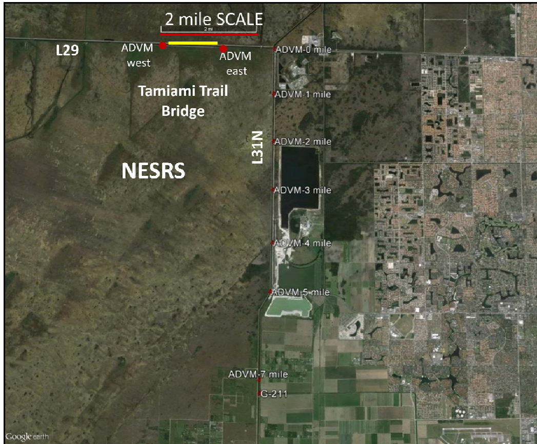
FIGURE C.1-5. EXISTING SURFACE WATER FLOW VELOCITY MONITORING ALONG L29 AND L31N WITH ADVMS
