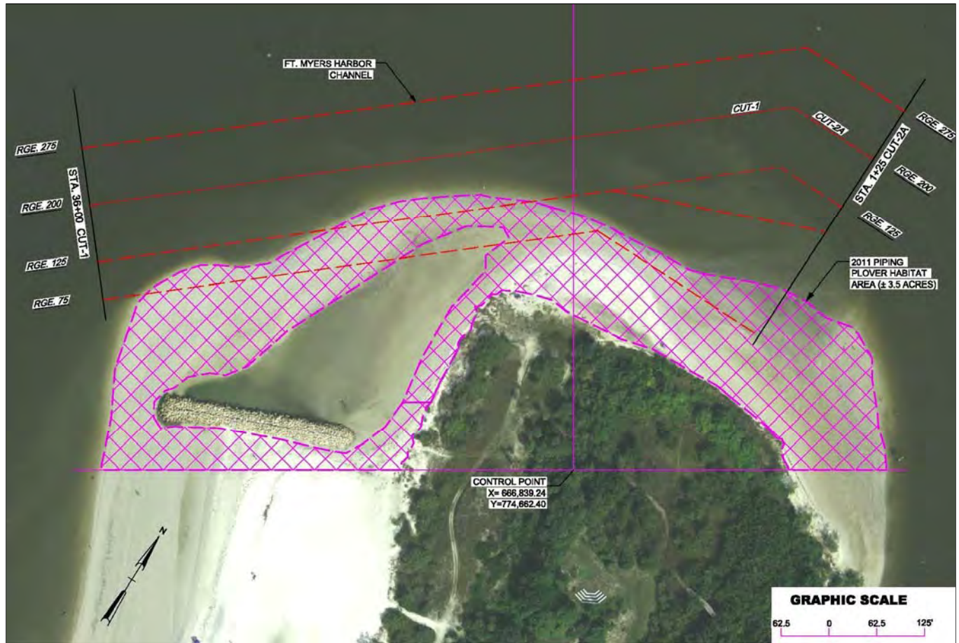
Figure 3. Bowditch Point after construction of the terminal groin and beach re-nourishment project, Lee County September 2011 (Note the intertidal pools to the left and right of the point, creation of additional beach, and extension of suitable piping plover habitat toward the northeast corner of the point).
