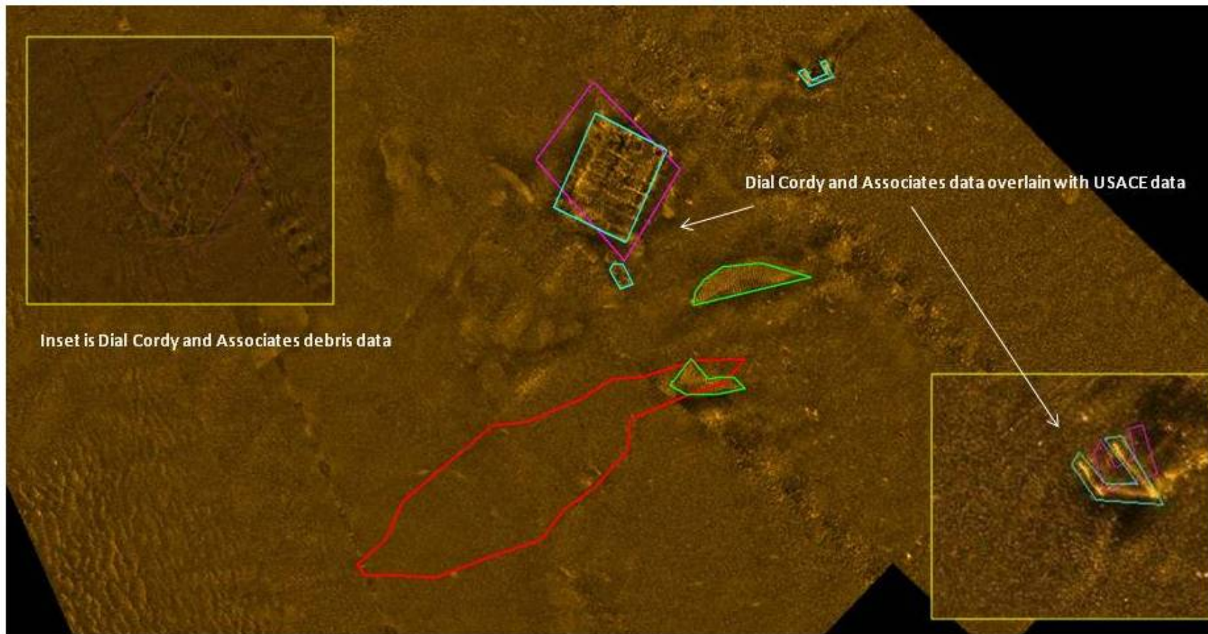
Figure 2-26: Hardbottom data from USACE survey geo-rectified with Dial Cordy Associates (DCA) data (August 2011). DCA data (red-lined polygons) are overlain by USACE Hydro-graphic Division data (green-lined polygons) on USACE collected sidescan data mosaic (August 2012). Note the absence of hardbottom features and presence of compressed sand and ripples.
