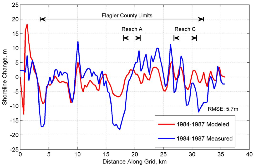
Figure A- 29. Final Calibration Modeled and Measured Shoreline Change
