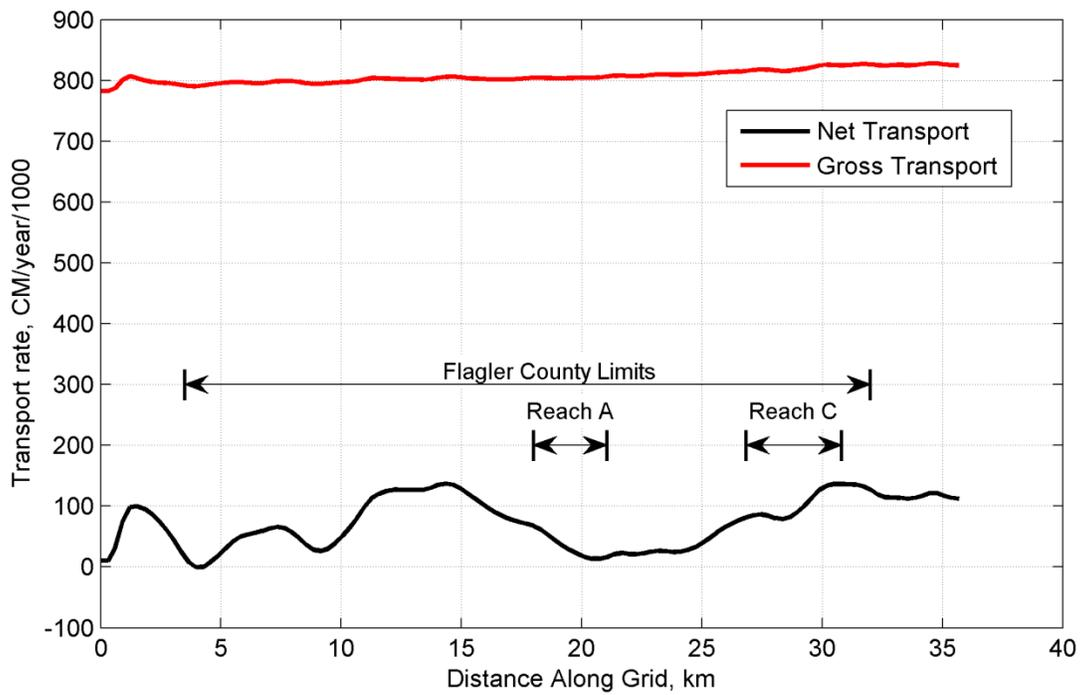
Figure A- 25. Longshore Sediment Transport for Calibration Run #1
