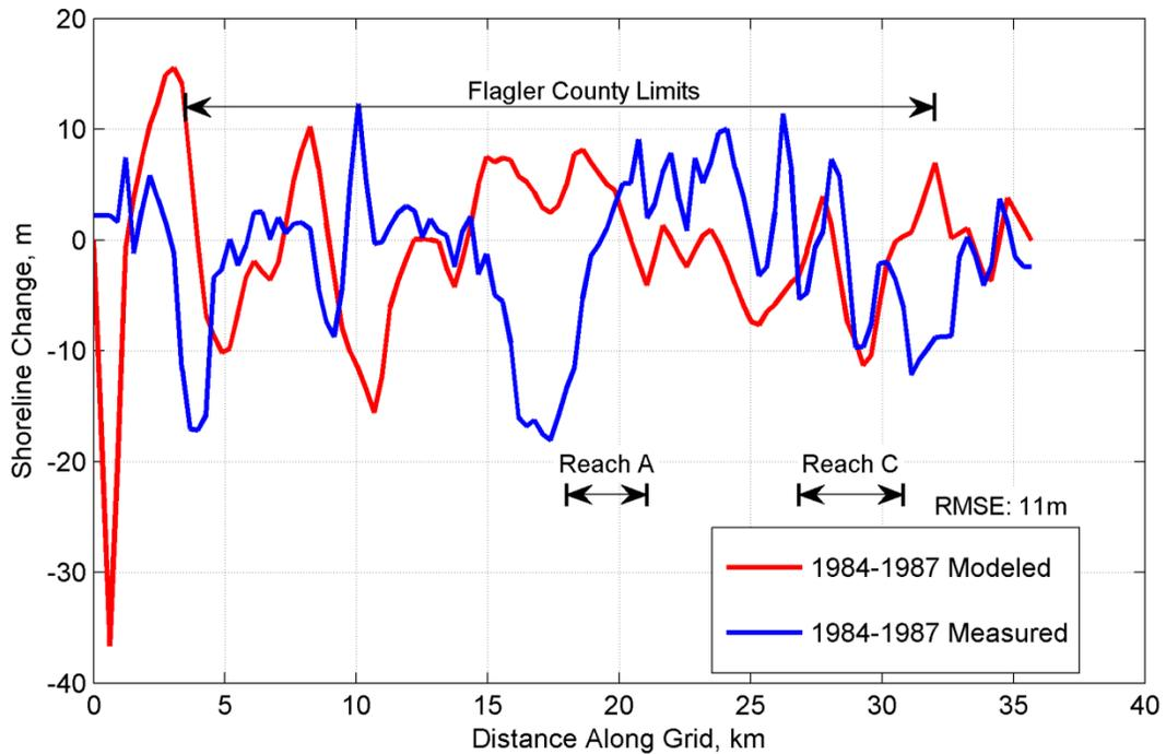
Figure A- 24. Modeled and Measured Shoreline Change during Calibration Run #1
