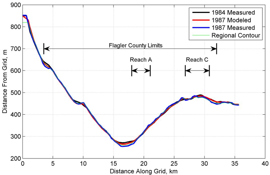
Figure A- 28. Final Calibration Modeled and Measured Shoreline Positions
