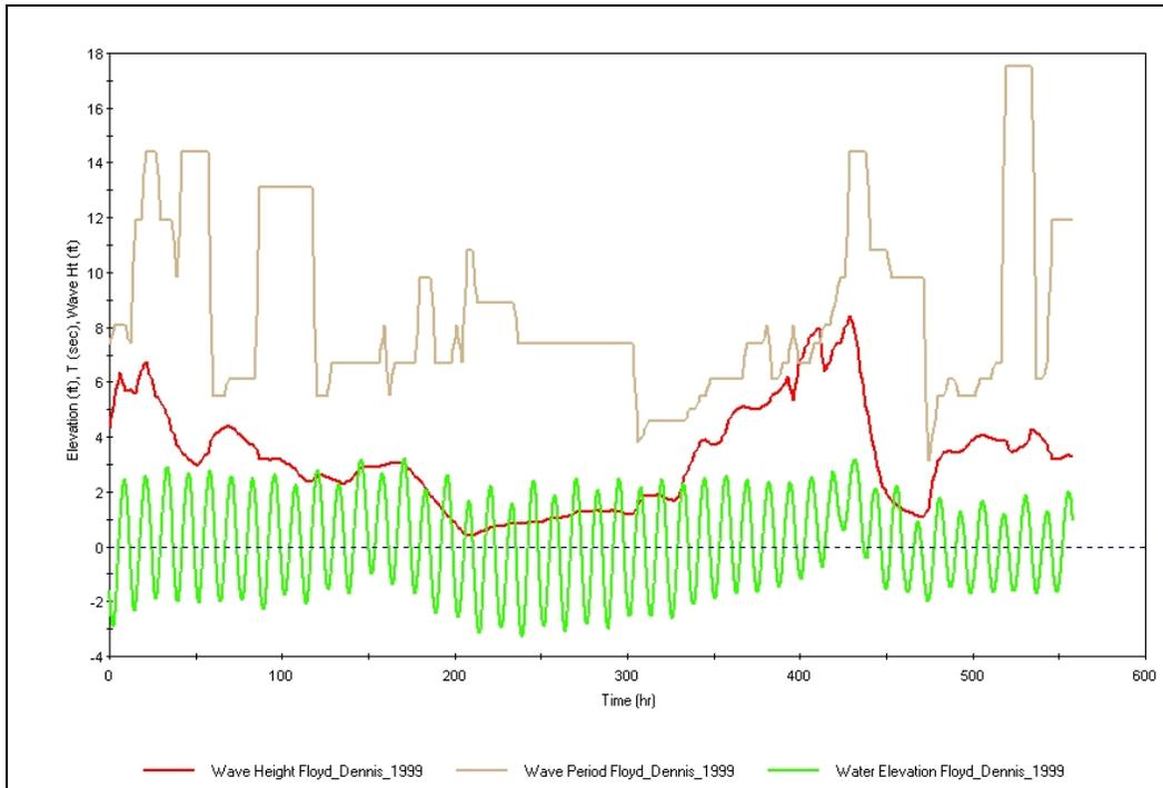
Figure A- 18. Hurricane Dennis and Floyd Wave and Water Level Data for SBEACH Calibration
