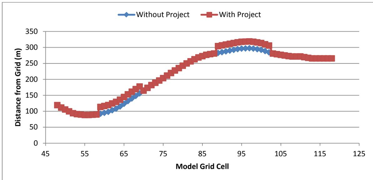
Figure A- 34. Initial model setup showing with and without project shorelines.
