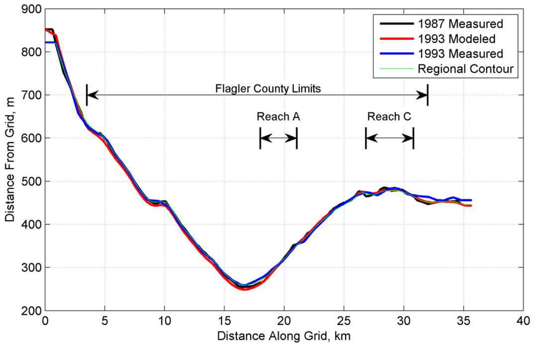
Figure A- 31. Verification Run Modeled and Measured Shoreline Positions
