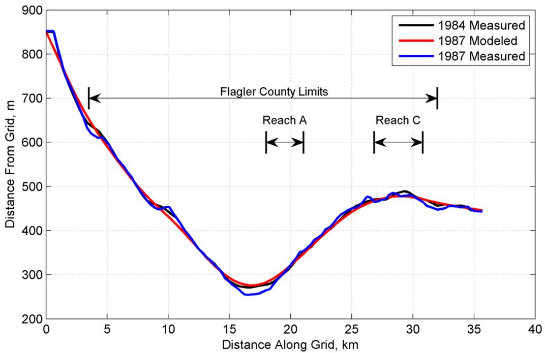
Figure A- 23. Modeled and Measured Shoreline Positions during Calibration Run #1
