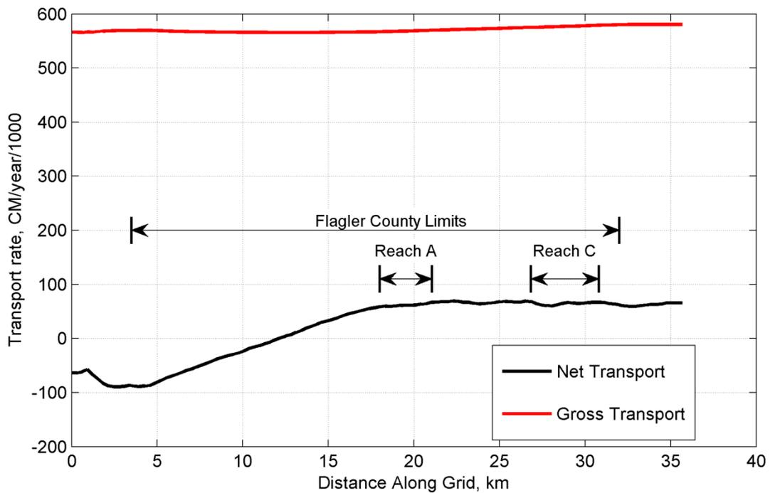
Figure A- 33. Verification Run Longshore Sediment Transport.
