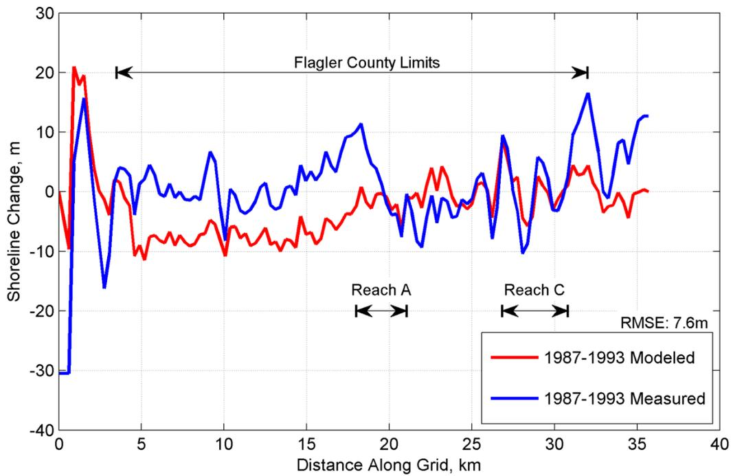
Figure A- 32. Verification Run Modeled and Measured Shoreline Change
