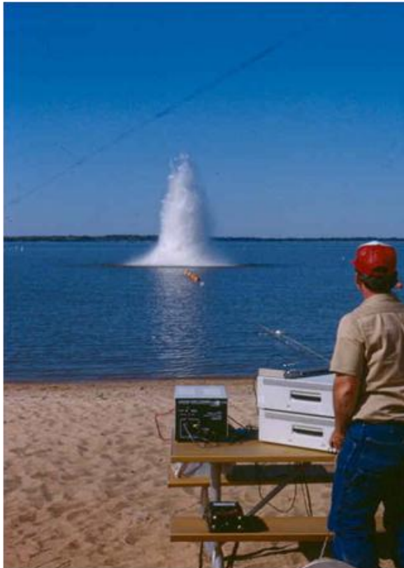
FIGURE 29: UNCONFINED BLAST OF SEVEN POUNDS OF EXPLOSIVES
