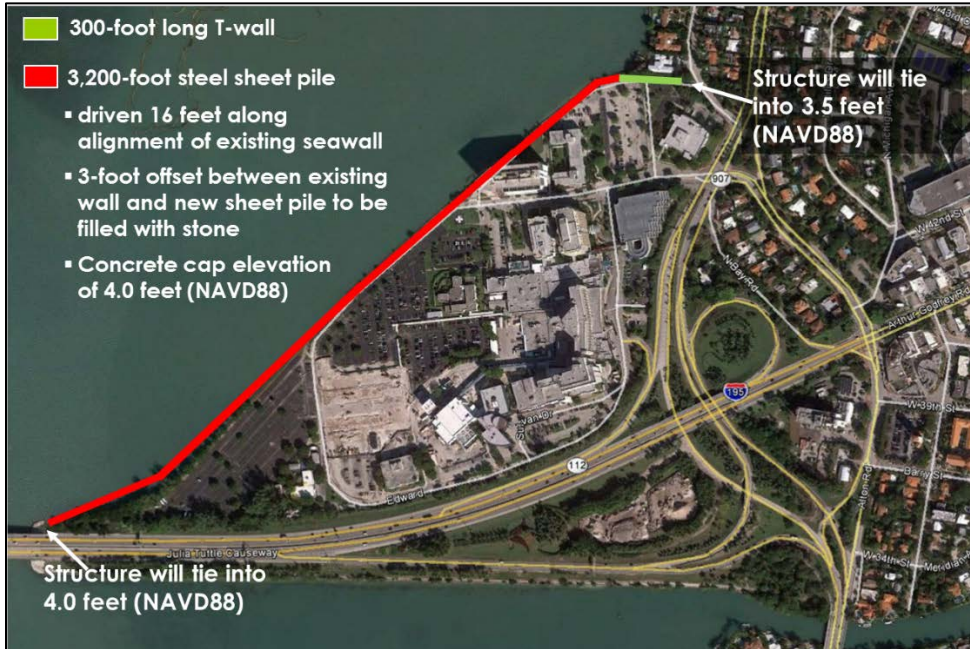
Figure 2.4 Alternative 1 (Sheet Pile Wall with T-Wall)
