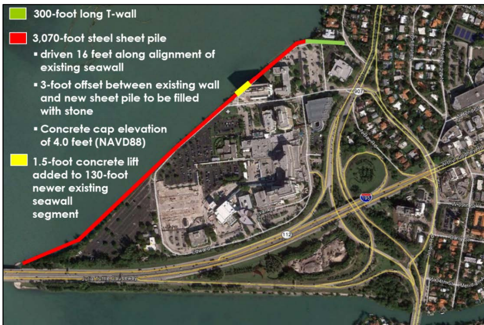
Figure 2.5 Alternative 2 (Sheet Pile with T-wall and Concrete lift)
