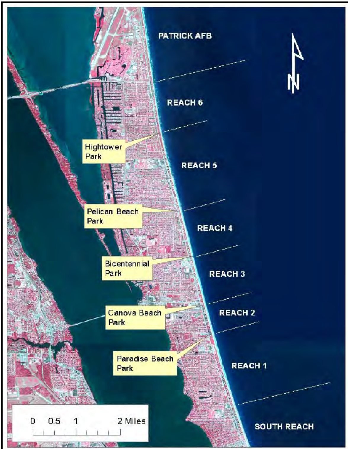
FIGURE 2: BREVARD COUNTY SHORE PROTECTION PROJECT MID-REACH SITE PLAN (SIX SUB-REACH SEGMENTS SHOWN)
