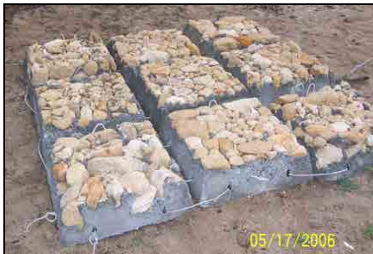
Figure 5. Sample portion of an articulated mat reef mitigation structure prototype proposed for the project.
