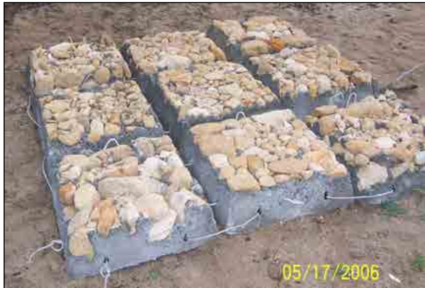
Photo 1. Sample portion of a prototype articulated-mat reef mitigation structure proposed for the project. Each block is about 30 in. x 30 in. x 12 in. (76 cm x 76 cm x 30 cm), with integral coquina rock surface. (The cable between the blocks illustrates the cable geometry that would be used in the articulated mat. Cable in the constructed materials would differ.)
