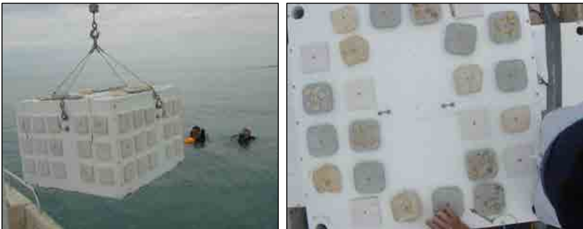
Photo 2. The PALM reef instrument deployed for Brevard County offshore of the Mid Reach is intended to measure Phragmatopoma caudata larval recruitment under different current regimes, chemical treatments, and macroalgal growth on four different types of substrates. 2a shows a photo of the Instrument platform being lowered into the water. 2b shows a photo of various substrate panels located on top of the PALM platform (Photos provided by K. Holloway-Adkins).
