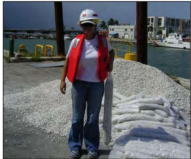
Figure 20: Stemming material utilized; bag is approximate volume of material used.
