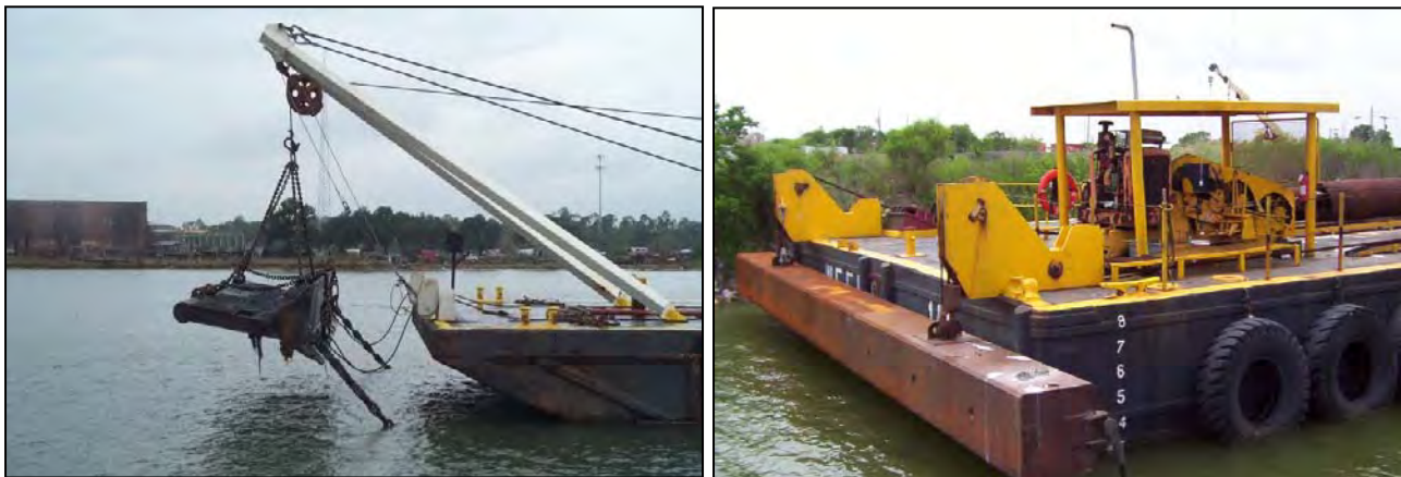
Figures 15 and 16: Example bed-levelers and associated operating conditions. Photograph courtesy: Bean Dredging Company and Weeks Marine Incorporated
