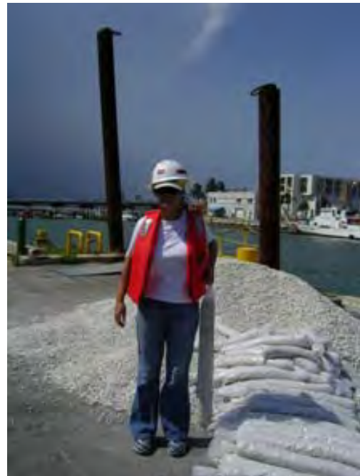
Figure 5: Stemming material utilized; bag is approximate volume of material used
