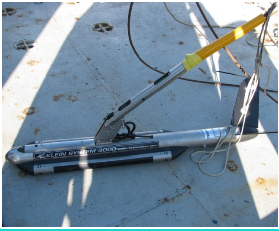
Sidescan sonar towfish is deployed to acoustically image seafloor
