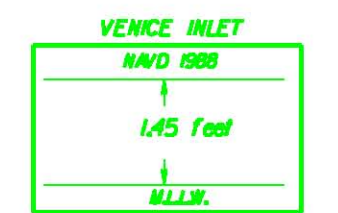
Relationship between NAVD 1988 and NOAA Mean Lower Low Water Tidal Datum (1983-2001) epoch
