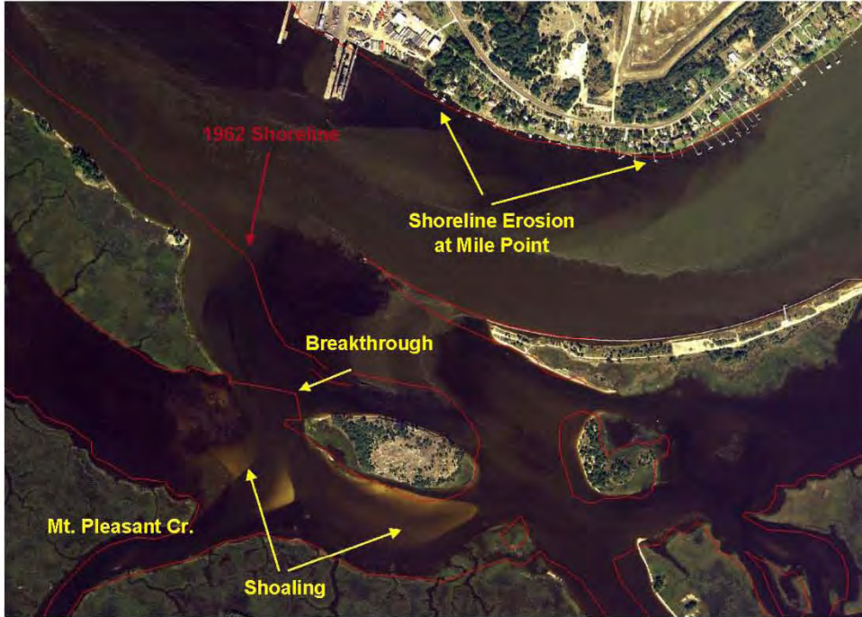
Aerial photo (2004) showing the change in river shoreline at Mile Point and Chicopit Bay since 1962. The erosion of Great Marsh Island's north shoreline continued until a breakthrough of the island occurred in the late 1990's.
