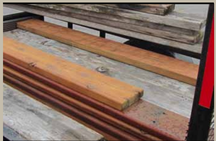
Volunteers re-plane and recycle old boards that are weathered and splintered, making them look like new. The boards are recycled and replaced on picnic tables, benches and other structures, saving both money and resources. (PHOTO COURTESY OF PHIL HART)
