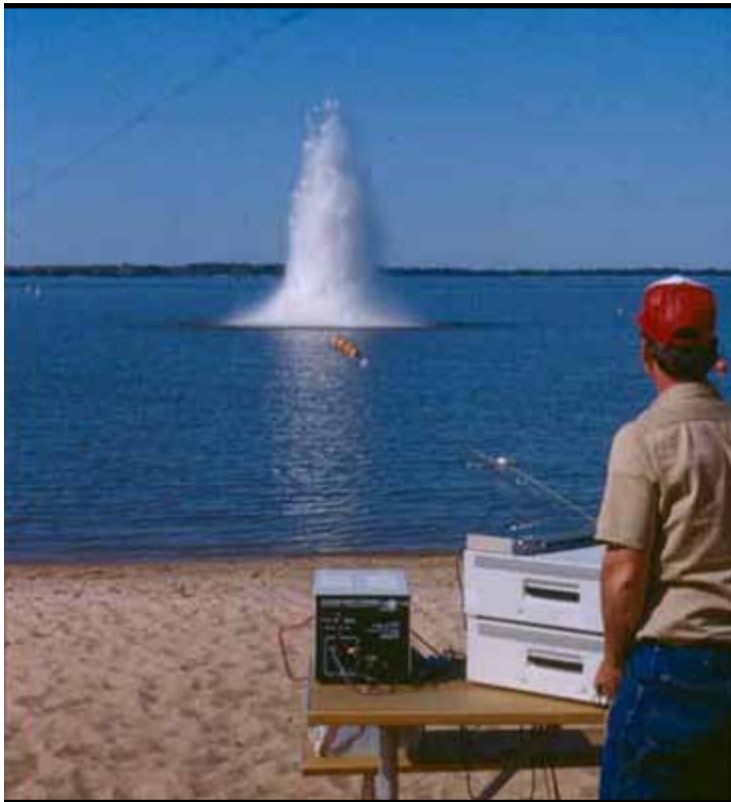
Unconfined blasting method, using seven pounds of explosives. (PHOTO BY TERRI JORDAN-SELLERS)
