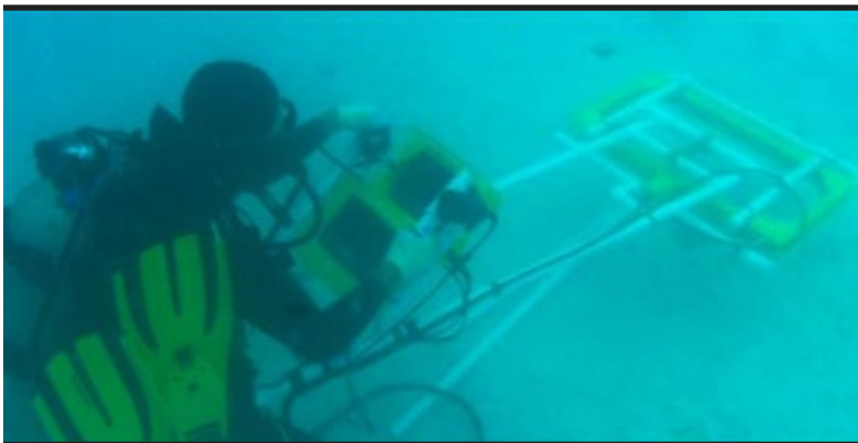
A diver uses an underwater digital geophysical magnetometer to locate potential munitions. (PHOTO COURTESY USA ENVIRONMENTAL)
