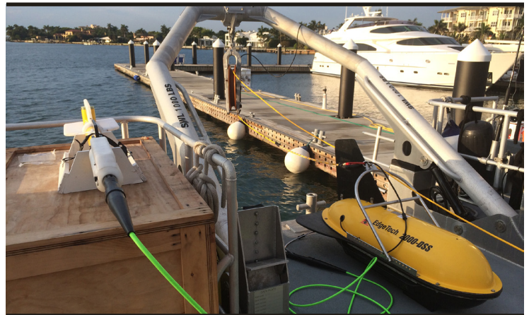
The large yellow capsule is the Edgetech 2000DS, which houses the side scan sonar and sub-bottom profiler. The side scan sonar sees the surface of the ocean floor and the sub-bottom profiler detects features just beneath the surface. Attached to this equipment via the green cable is the magnetometer, which is like a metal detector that picks up ferrous materials above and below the surface of the ocean floor, particularly ship hulls, ship elements, fittings, cannons, anchors and more.
