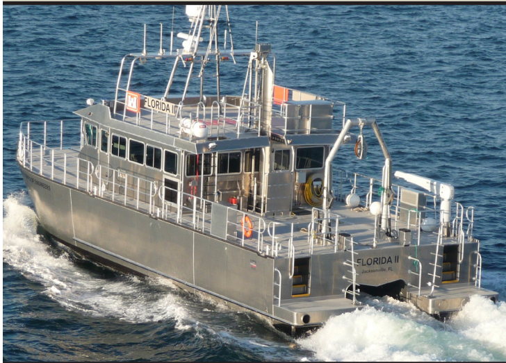
The Florida II, Jacksonville District's new survey boat, takes to the water as part of its final testing before delivery in 2013. The state-of-the-art vessel can collect data at depths of 30 to 1,000 feet and has a top cruising speed of 36 knots. (Photo courtesy of All-American Marine)
