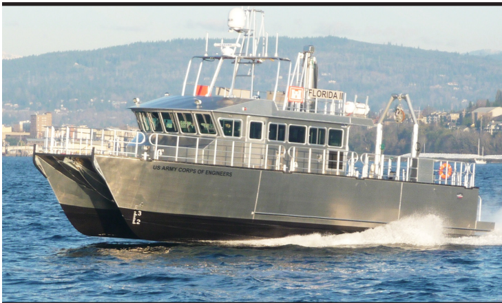
The Florida II cruises up to 36 knots when under way, moving quickly to the next job. Much of the hull is out of the water at higher speeds, thanks to the assistance of a fixed hydrofoil mid-ship. (Photo courtesy of All American Marine).
