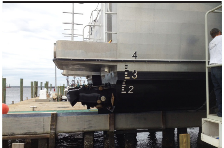
The jet propulsion system (rather than a rudder and propellers) provides improved maneuverability. Even docking is simple; the vessel can move sideways with one movement of the joystick. (Photo by Phillip Bates).
