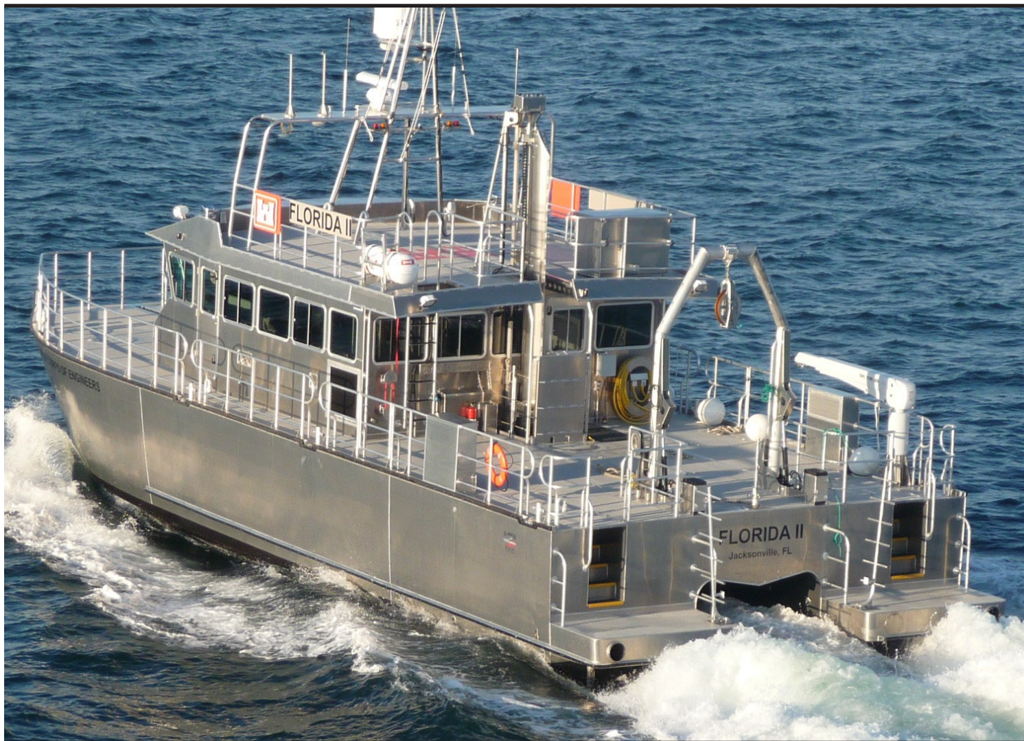
The name on the transom says it all: the Florida II hails from Jacksonville, Fla. The A-frame on the stern is used to deploy sonar towfish capable of collecting data at depths of 30 to 1,000 feet, as well as specialized data such as the presence of metals. (Photo courtesy of All American Marine).
