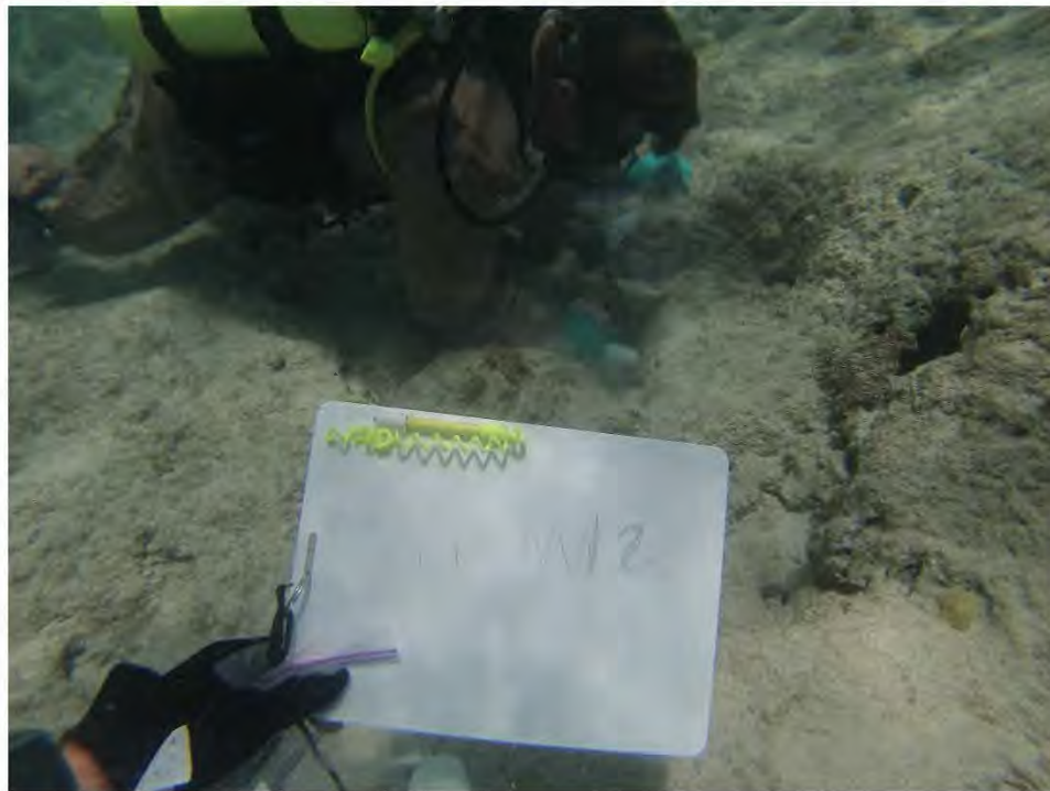
Figure 4-7: UXO Technician SCUBA Diver Collects a Discrete Marine Sediment Sample (ITEM 12/Sample number PR-1404-SDM-13-14A was moved to collect the sample)
