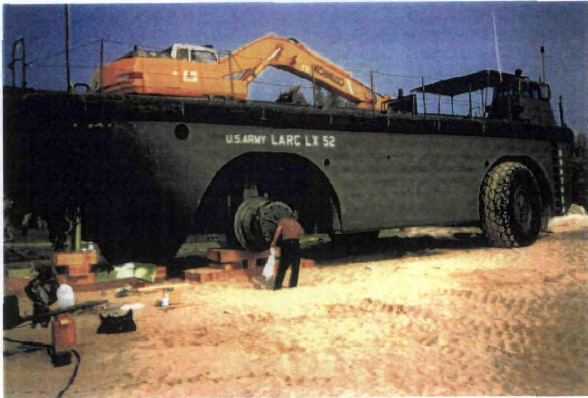
Changing damaged tire on LARC 52 at Round Island Park by 309 th Transportation Unit Personnel.
