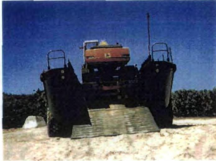
Track hoe mounted on platform in well deck of LARC 52. Bow ramp down for clarity.
