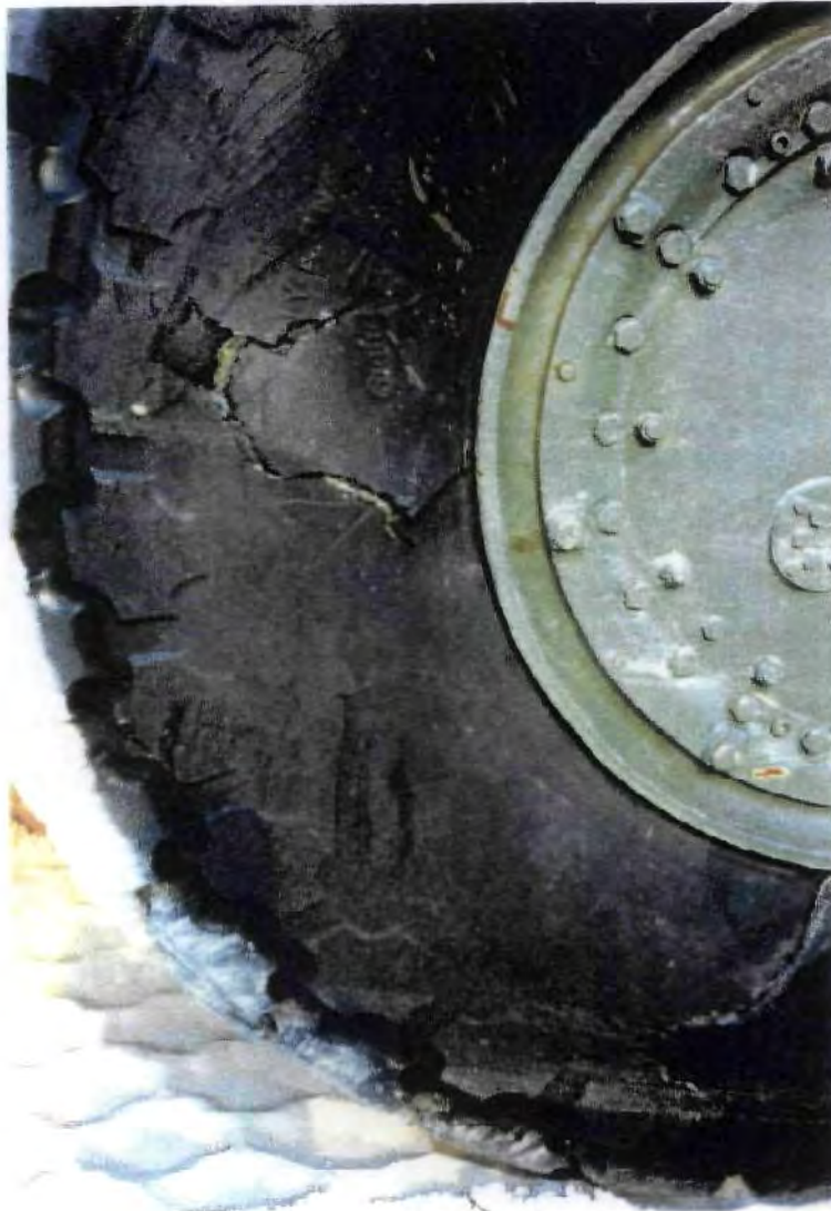
Damaged tire on LARC 52 caused by underwater Obstacles.
