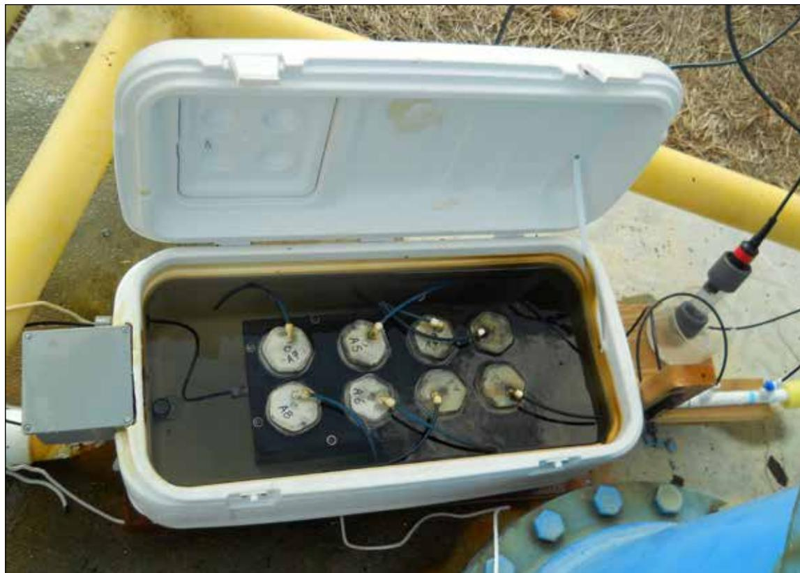
Figure 1-15. The above ground flow through microcosm in the field.
