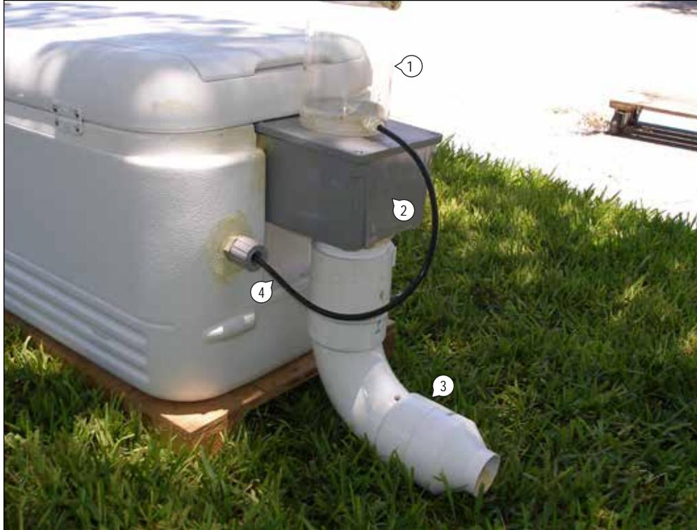
1. Multiprobe flow cell for monitoring pH, temp, ORP of GW leaving the SS flow-through chamber
