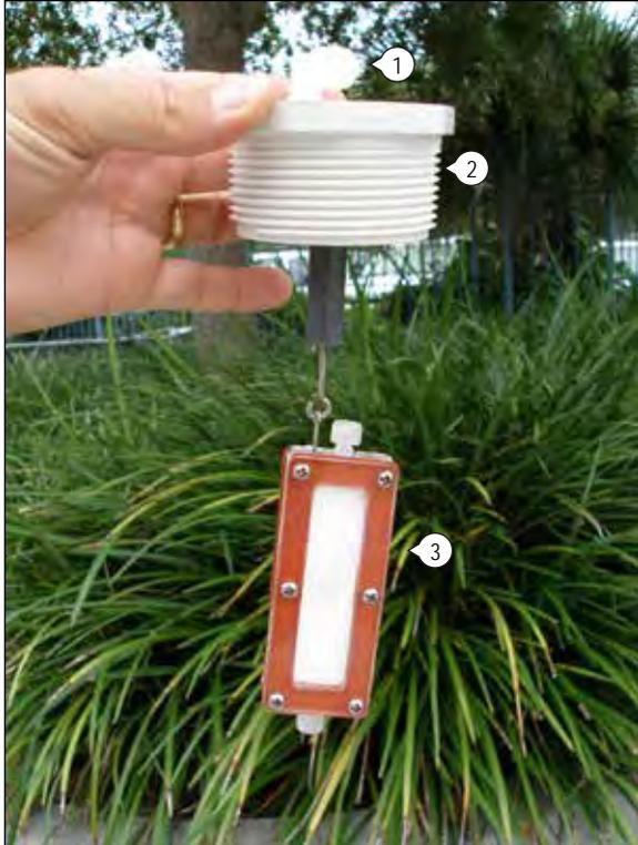
1. Off gas release fitting that allows gases released within the stainless steel (SS) flow cell due to depressurization to vent into the water jacket
