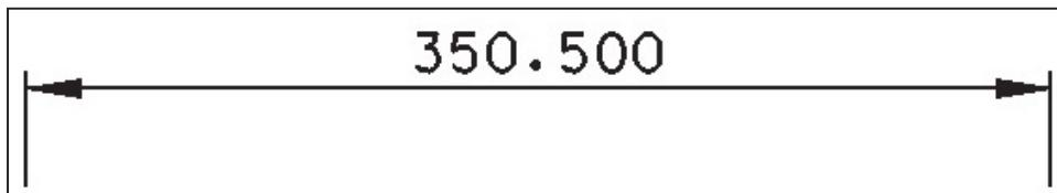
Figure 3-12. Dimension in meters. Always shown as a real number (with decimal).
