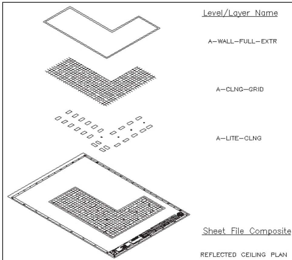
Figure 4-1. Typical levels/layers contained in a sheet file.
