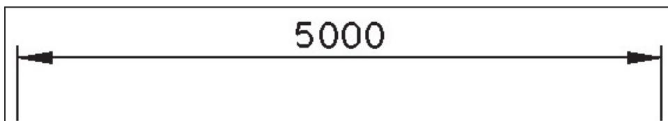
Figure 3-13. Proper dimension presentations for metric measurements with four or fewer digits.
