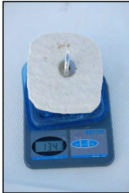
Figure 2-4 Block of plaster of Paris on scale showing hardware used for deployment.
