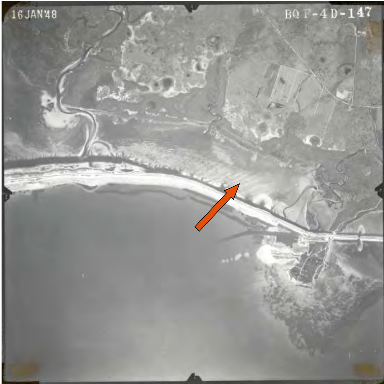
Figure 4 Aerial photograph from 1948 showing apparent impacts to seagrass meadows north of the CCC at the eastern terminus of the causeway. The red arrow indicates the photographic signature of shallow areas devoid of seagrass.
