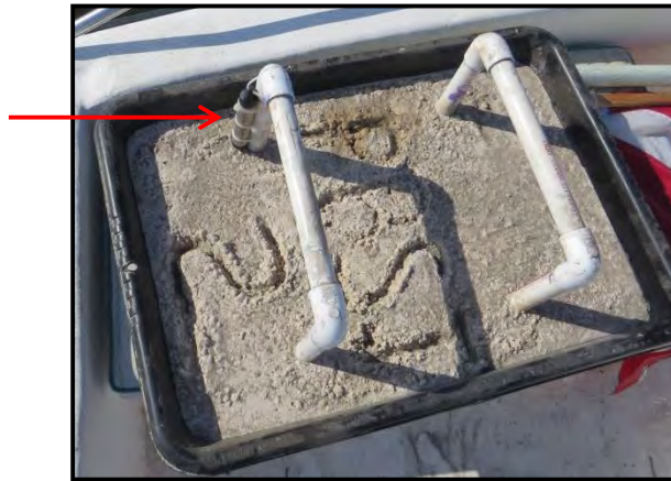
Figure 2-2 Solinst Levellogger (indicated by red arrow) attached to concrete base.
